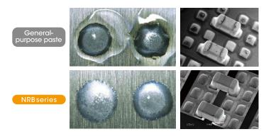
Void-free soldering with NRB60 and SVR-625GTC
