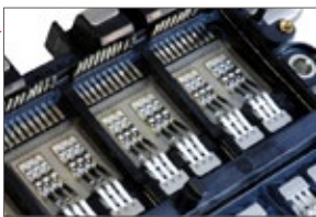
Power semiconductor mounting using preform with Ni balls
