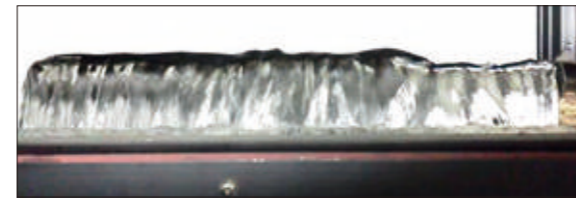
従来偏流板 With a conventional deflecting plate
