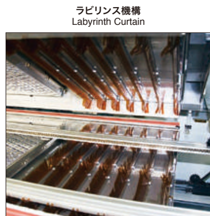
外気の流入及びN 2 雰囲気の流れ抑制 Prevents inflow of outside air and outflow of N 2 atmosphere
